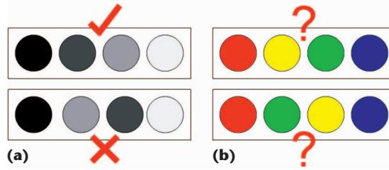
**1 Perceptual ordering.** (a) We can easily place the gray paint chips in order based on perception, (b) but cannot do this with the colored chips.
