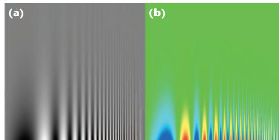
**2 Spatial contrast sensitivity function.** Frequency increases to the right and contrast increases toward the bottom of both images in the figure. We can see detail at much lower contrast in the (a) luminance-varying gray-scale image than with the (b) rainbow color map.
